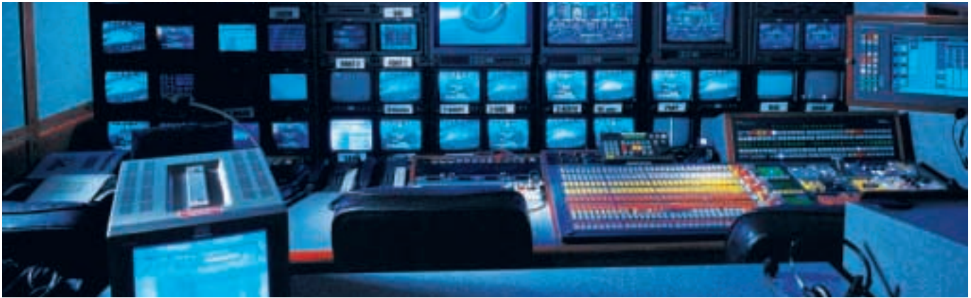
■ An NEP outdoor broadcast van featuring a Grass Valley Kalypso Video Production Center Switcher
