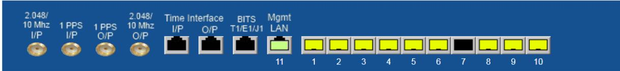
In this example all ports are connected except #7, the top QAM port.
